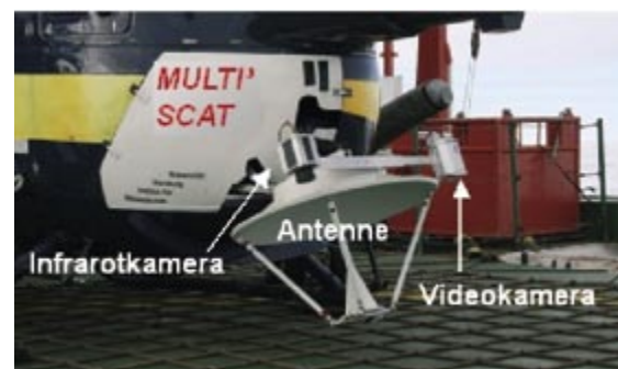
Radarantenne, Infrarot- und Videokamera des Multi3Scat. Radar antenna, infrared- and video camera of the Multi3Scat.
